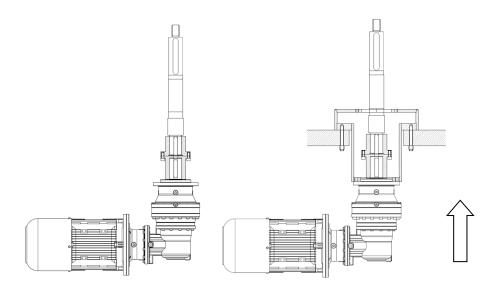
3. From the top fix the bearing and seal holder on the base. insert the chainwheel spacer on the shaft in its position
