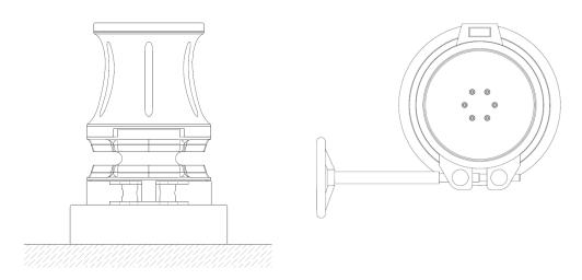
ATTENTION: Apply grease to the main shaft and on each screw before fit all the parts
