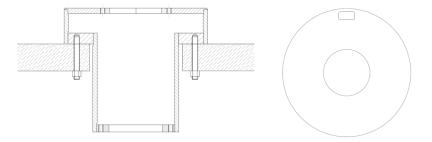
2. Fix the supplied screwed bush on the top of the main shaft and use it to lift the motor-gearbox from the chain locker into the base in the needed position. Fix it by n.10 M12 screws.
