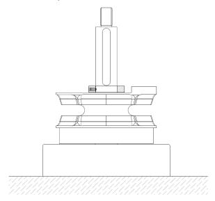
5. Insert the drum and screw completely the top cap. Insert the band brake with brake stopper seat on the brake stopper block
