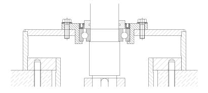
4. Insert the chainwheel on the shaft and block it by the stopper spacer. Screw the three nuts. Check that the chainwheel is free to rotate. Insert the key on its seat on the shaft
